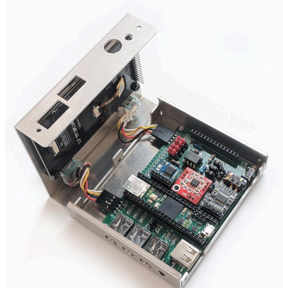
Align both enclosure parts together. Attach the encoder connectors to the MDT PCB.
