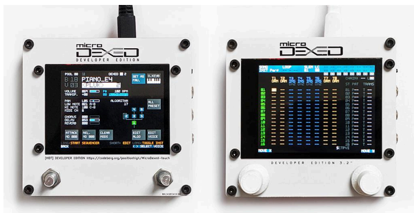
(PCB BASED FRONT/BACK PANEL, DISPLAY SIZE LEFT 2.8" and RIGHT 3.2")
