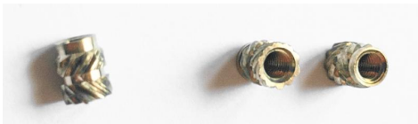
These are the inserts we are using, the M3 x 5.7 x 4.6
