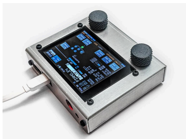
MDT (Metal enclosure) with the 12mm (low height) encoders
