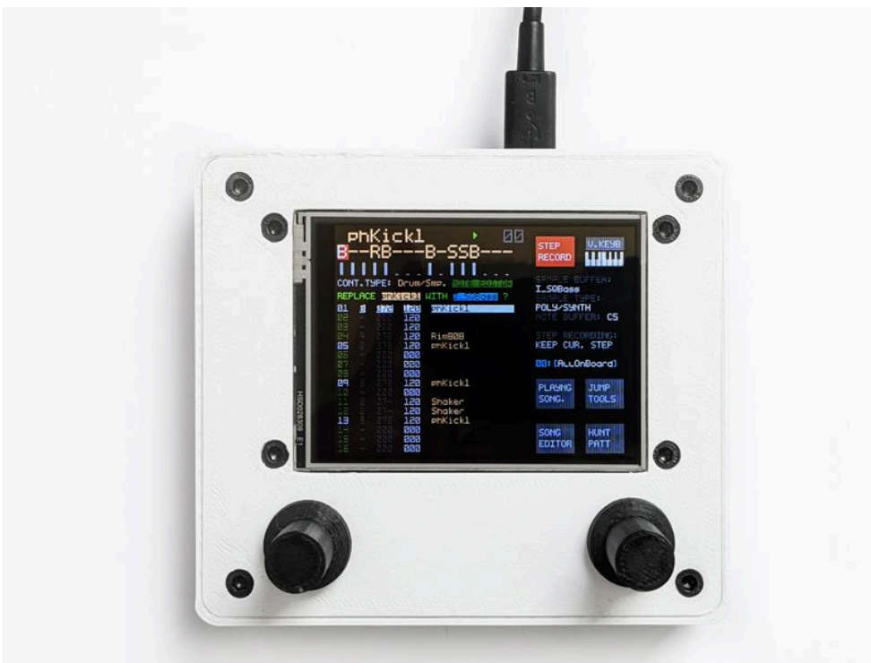
MDT (first gen) with 2.8" display and self printed FDM case
