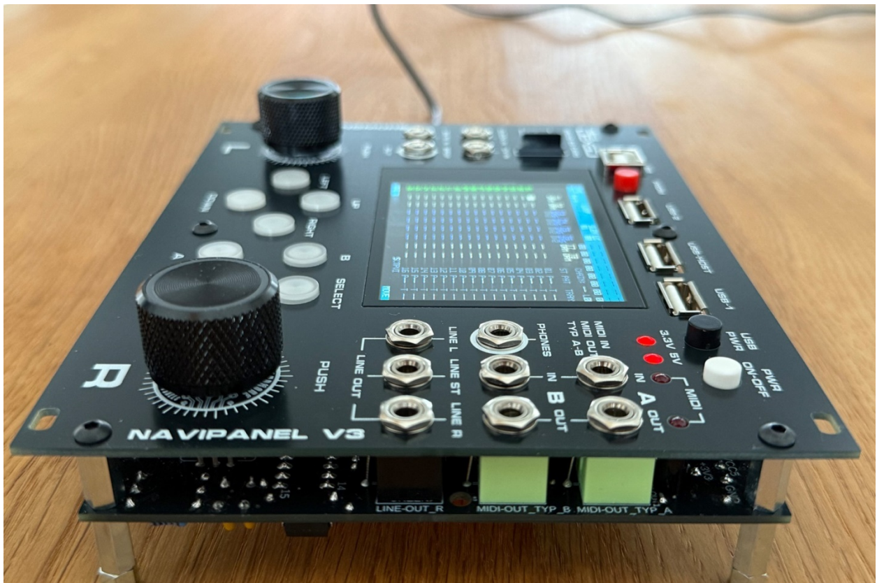
Example: Finished device the TFT display must be flush with the front panel
