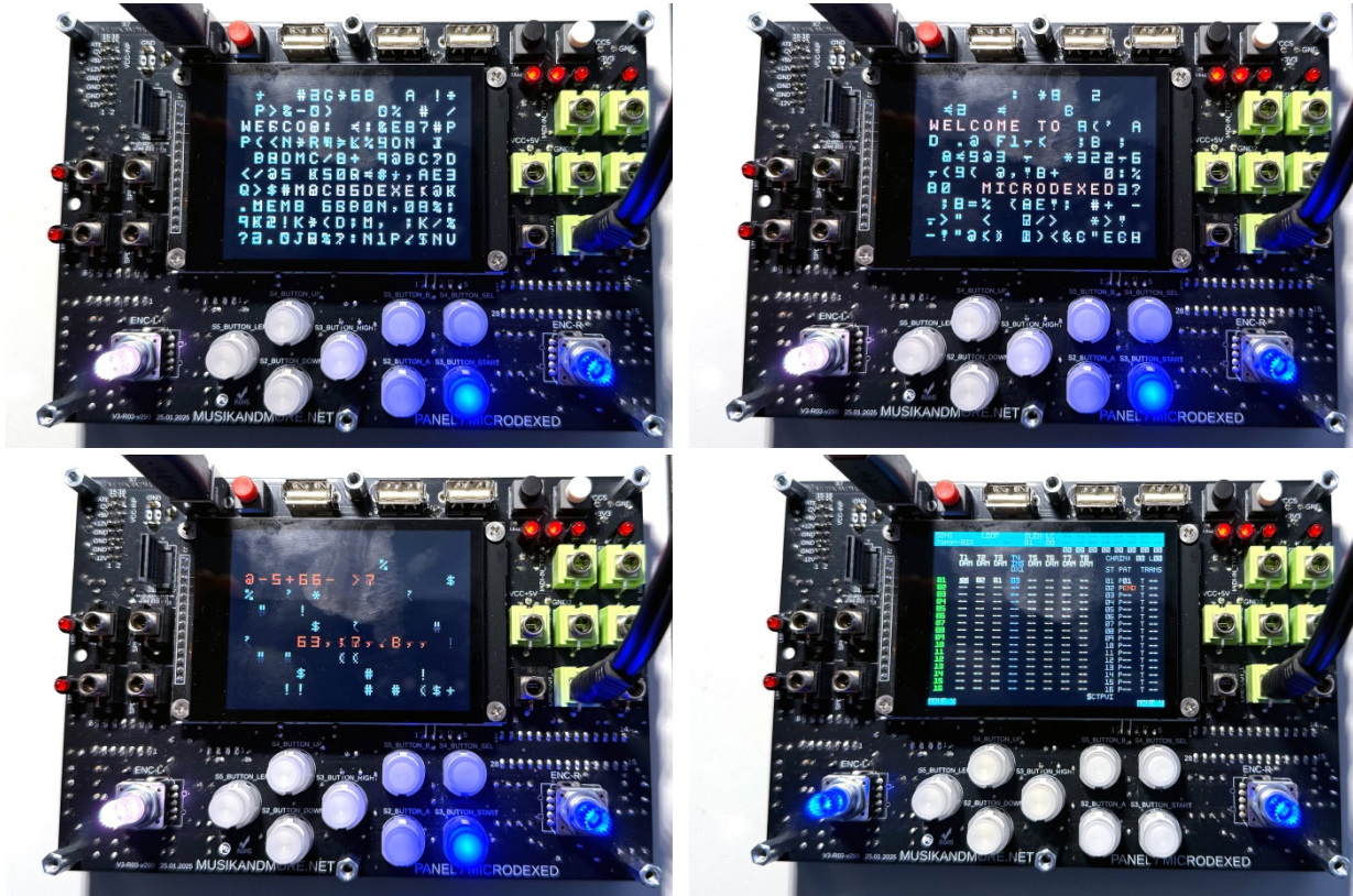
Mainboard boot process with LED test and start screen
