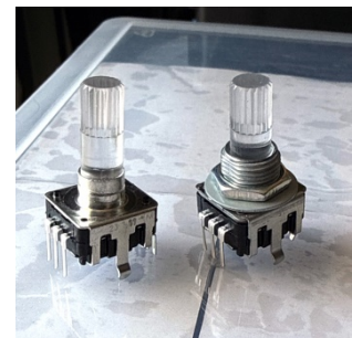
RGB rotary knobs 22mm installed in the front panel - Knobs with RGB encoder Left: Encoder without thread
