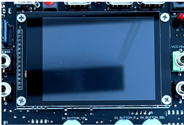
Insert TFT and fix with SK M3x4
