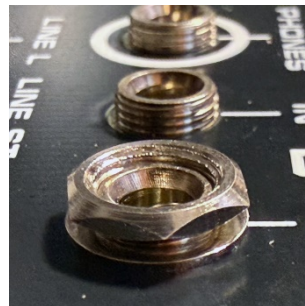
3. 1x M6 hexagon nut for all 12 TS/TRS sockets
